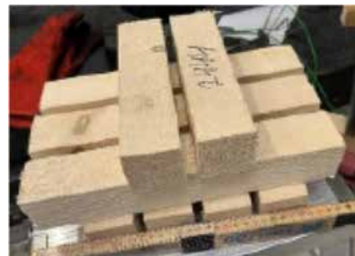
Placement of the fuel load in the firebox
